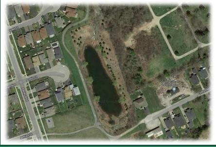
A stormwater management facility is a man-made infrastructure built to gather rainfall and surface water runoff. Stormwater runs off of our roads, driveways, sidewalks and throughout our community collecting dirt, litter and other pollutants before draining into the stormwater facility. Sand, dirt, silt and other sediments that pollutants attach themselves to settle to the bottom of the facility. Cleaner water leaves the stormwater facility and flows into our watercourse.
